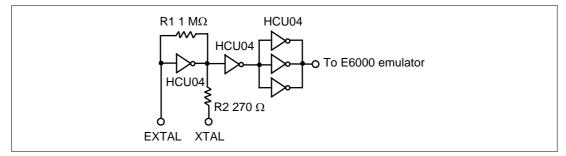
Figure 10 Oscillator Circuit
